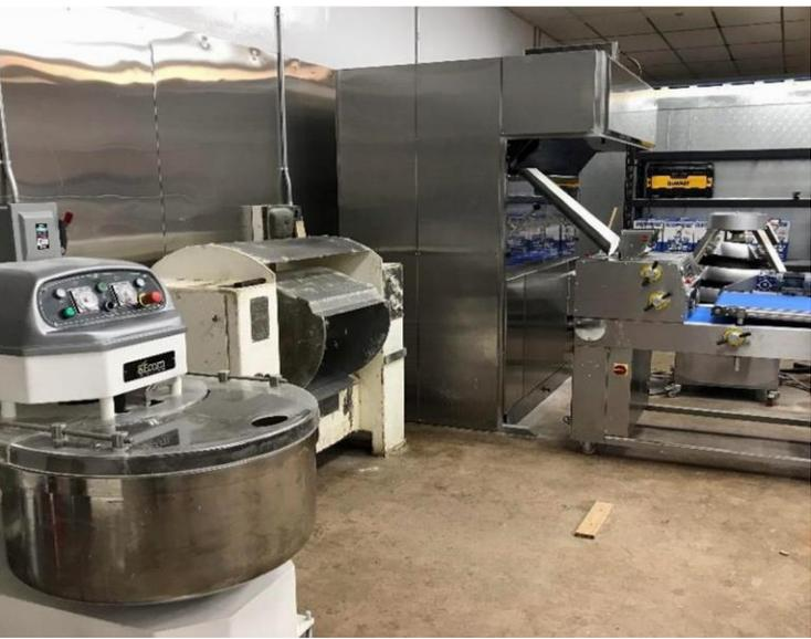
**The new line including the divider, rounder, proofing cabinet and sheeter.**
